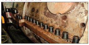
Applications set into a pocket or a counter bore situation pose a problem with conventional tooling. Standard drive extensions and machined down accessories compromise the safety of the operator! The design and the mechanics of the HYTORC Nut™ allows positioning of the torque wrench away from the conflict area!
